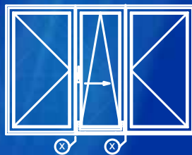
Schematic: G Fixed / Sliding / Fixed Turn* / Sliding / Turn*
